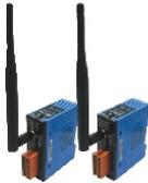
6 Digital Input Channels and 4 Relay Output Channels
