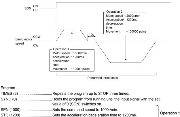
MOV (12000) ...... Executes movement by 12000 pulses in the CCW direction.
