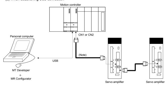
Note. Q173HCPU: 2 systems (max. 32 axes), Q172HCPU: 1 system (max. 8 axes)
